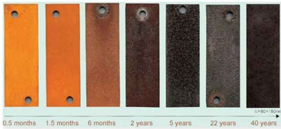
Weathered steel color progression over time. Photo provided by Eversource.
