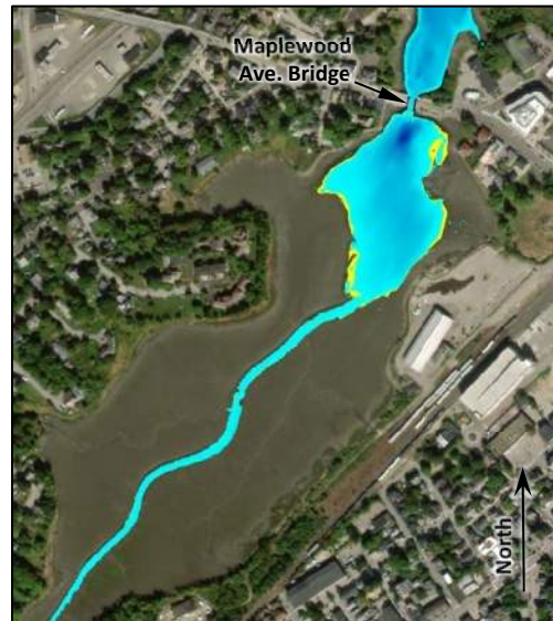
Figure 33 – Inundated areas at the MLLW tide stage trough with 1.0 ft SLR. Blue shading represents the post-project inundation area and yellow shading indicates the additional areas inundated under pre-project conditions
