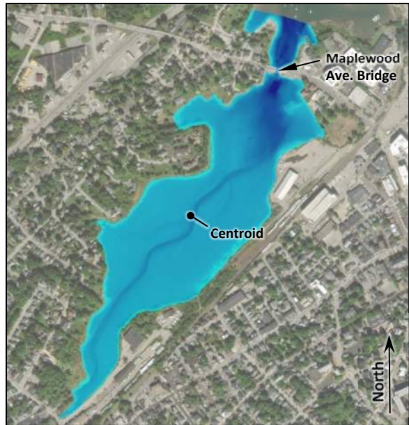
Figure 14 – Inundation area at the MHHW tide stage crest and centroid of the portion of North Mill Pond south of Maplewood Avenue
